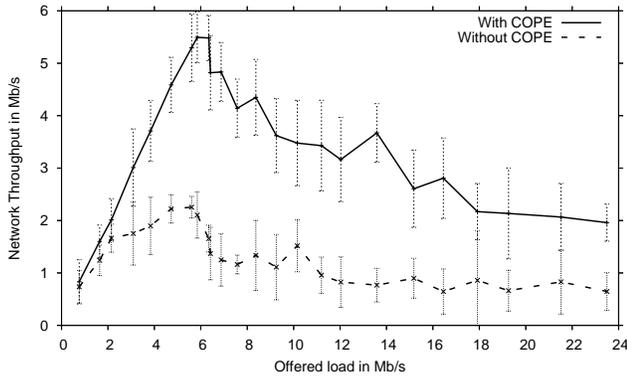
**Figure 12**—COPE can provide a several-fold (3-4x) increase in the throughput of wireless Ad hoc networks. Results are for UDP flows with randomly picked source-destination pairs, Poisson arrivals, and heavy-tail size distribution.
