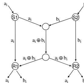
**Figure 2**—A simple scenario showing how network coding improves throughput. All links have a capacity of one message per unit of time. By sending the XOR of  $a_i$  and  $b_i$  on the middle link, we can deliver two messages per unit of time to both receivers.
