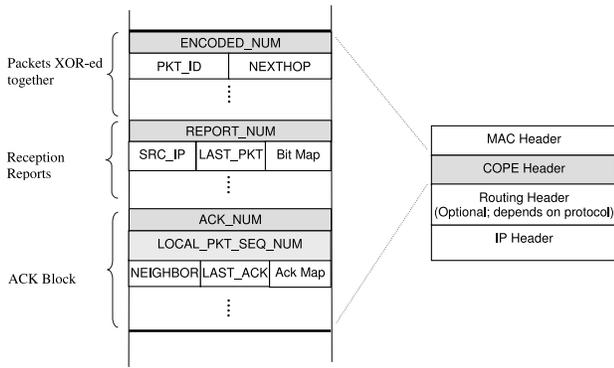
**Figure 5—COPE Header.** The first block identifies the native packets XOR-ed and their nexthops. The second block contains reception reports. Each report identifies a source, the last IP sequence number received from that source, and a bit-map of most recent packets seen from that source. The third block contains asynchronous acks. Each entry identifies a neighbor, an end point for the ACK map, and a bit-map of ack-ed packets.
